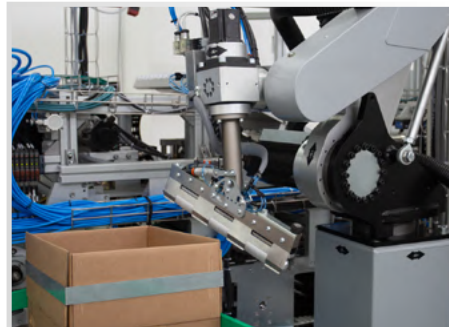
Robotic feeding system for empty capsules
