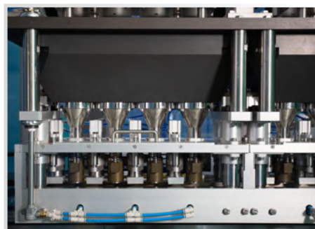
Innovative system for capsule filling, pressing and cleaning
